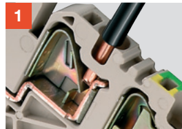
1 View without housing side plate
